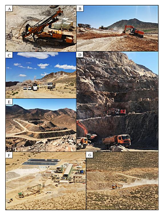
Figure 2. Illustration of some mining activities, Jbel Tirremi project, Morocco; A) exploration (drilling and boreholes); B) access tracks; C) blasting; D) open pit method (drilling and loading);
